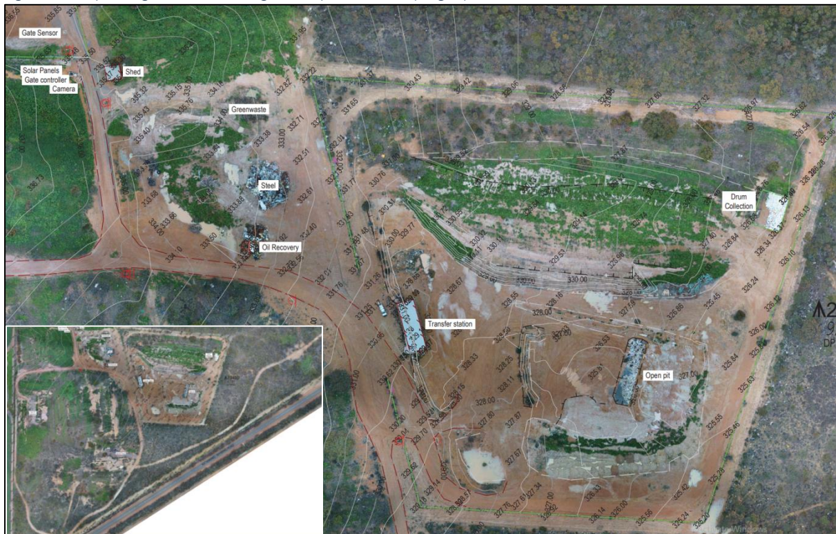
Figure 2.1 Nyabing landfill existing site layout and topographic contours
